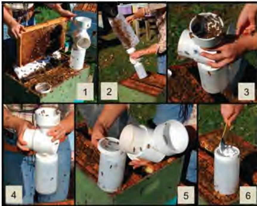
Figure 3. Gizmo, a device that can be used to measure 300 adult bees by volume. To operate 1) shake a frame of bees onto a piece of flashing (or cardboard, newspaper, election sign, etc.) as long as a frame and bent into a V-shape, then 2) dump the bees into the top of Gizmo. 3) There is a volume inside Gizmo that measures 300 bees. 4) Rap Gizmo onto a hard surface three times, then turn the handle to release the bees into the jar. 5) Remove the jar and screw on the mesh lid, then 6) add powdered sugar to dislodge the mites.
