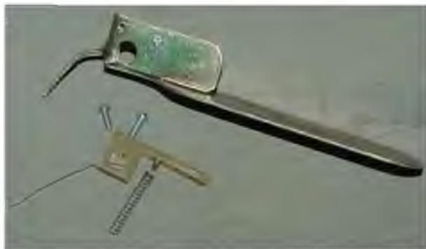
Figure 7. The grafting tool disassembled.
