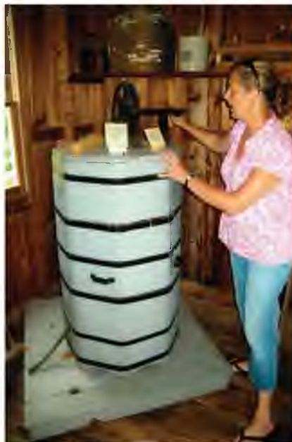
A wooden barrel extractor with a planetary cast iron hand operated gear drive is a highlight of the honey house.
