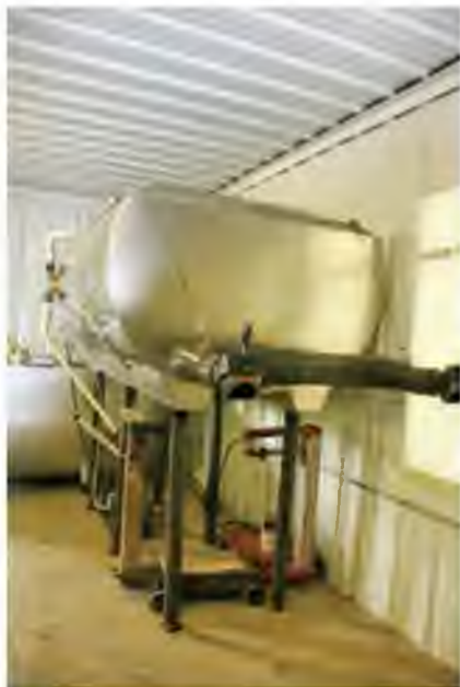
Their bulk honey tank holds 15 barrels of honey. From the large flow spouts they can fill a 55 gallon drum in ten seconds.
