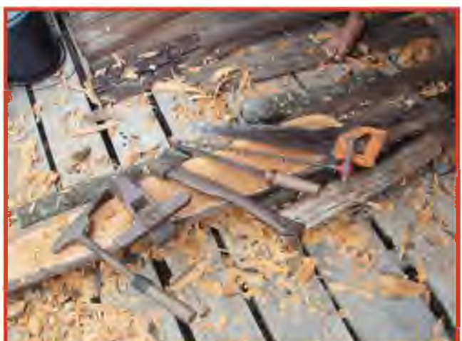
Simple hand tools are all that are available for tikung construction. Below from left to right — adze, plane, hand-axe, rasp, auger, and handsaw.
