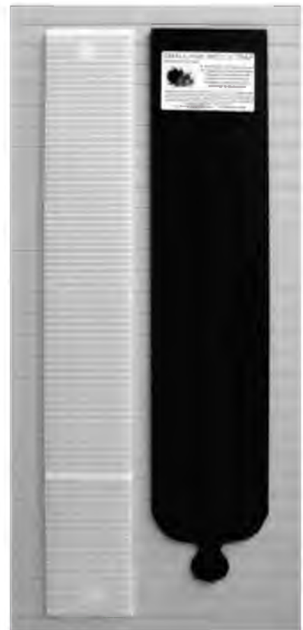
Figure 2: Both types of d-strips, which efficacies were compared in the test: Transparent (original) d-strip (left; 75’500’4 mm) and black d-strip (right; 100’478’4 mm).
