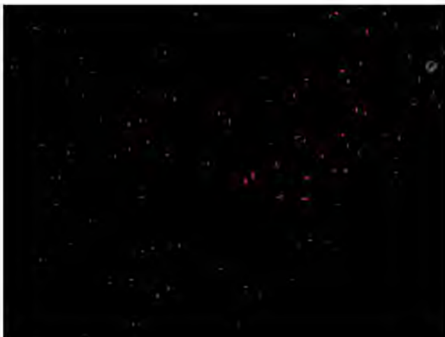
Fig. 5. The spores that glow red under UV light are not viable. The spore membranes have been ruptured by a sterilizing agent, and a red fluorescent stain has penetrated these spores.
