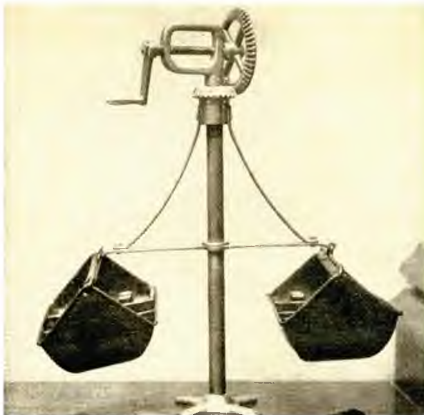
Adair's "Meliput" weighed 28 pounds and sold for $14. He claimed it would empty the honey with half the motion needed for any other since the cells of the comb were always in line with the motion. It was sold during the period of 1869-1872.
