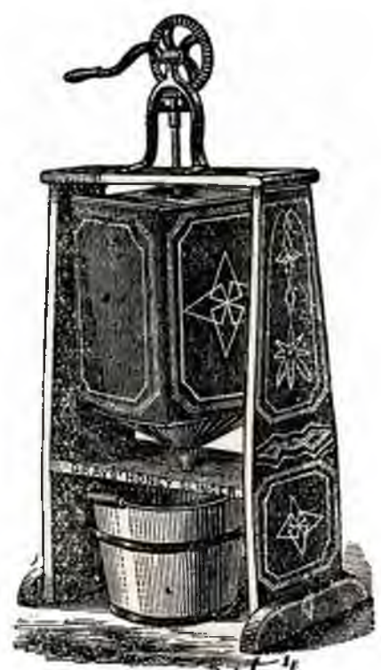
"Novice's" (Root's) improved metal can with faucet. At right, Gray's Honey Slinger with vertical crank.
