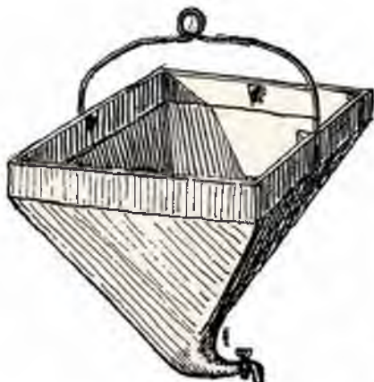
The first extractor. Hruschka’s smelatore swung at the end of a rope.
