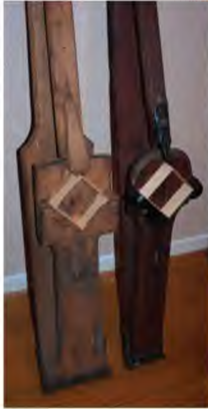
Figure 7. Section presses. Note the section box in either mount. Pushing it forward brought the upper piece down slightly to lock the top corner. The press on the left is the original. The other was a later version mass-produced by the A. I. Root Company, once a large beekeeping manufacturing company.
