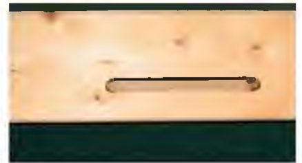
The entrance is cut with a router at an angle, so rain can't enter the hive.
