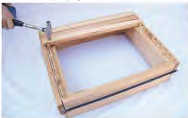
(l) Photo 5: A frame nailing jig setup with end pieces and wedge top bars. Use PVA glue on the end pieces, tap in place with a tack hammer and nail the top bar with long clay coated frame nails. (r) Photo 6: Use the Clamp-It® system to square up the bee box before joining the glued countersunk sides with deck screws.
