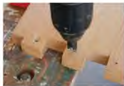
Photo 2: Use a combination countersink drill bit to prepare the bee box for the screws. The countersink makes it easy to do two jobs at once—drill a pilot hole, (if needed), as it whittles a neat circle to create a well for the screw head.
