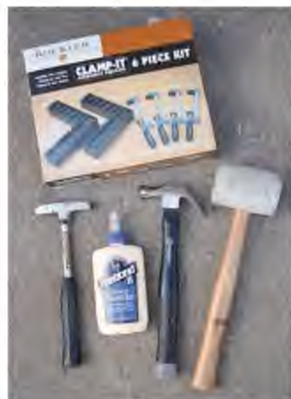
Photo 3: Clamp-It® System, tack hammer, PVA glue, claw hammer and a rubber mallet are some of the necessities for assembling bee equipment.
