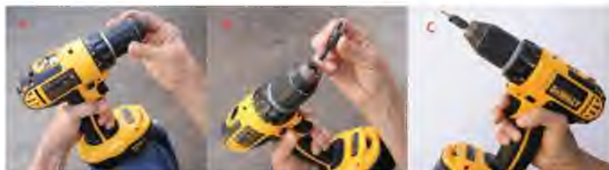
Photo 1 A: Rotate the keyless chuck to the right. 1 B: Insert the countersink, drill bit or hole saw. 1 C: Rotate the chuck to the left to tighten. The drill is ready to use.
