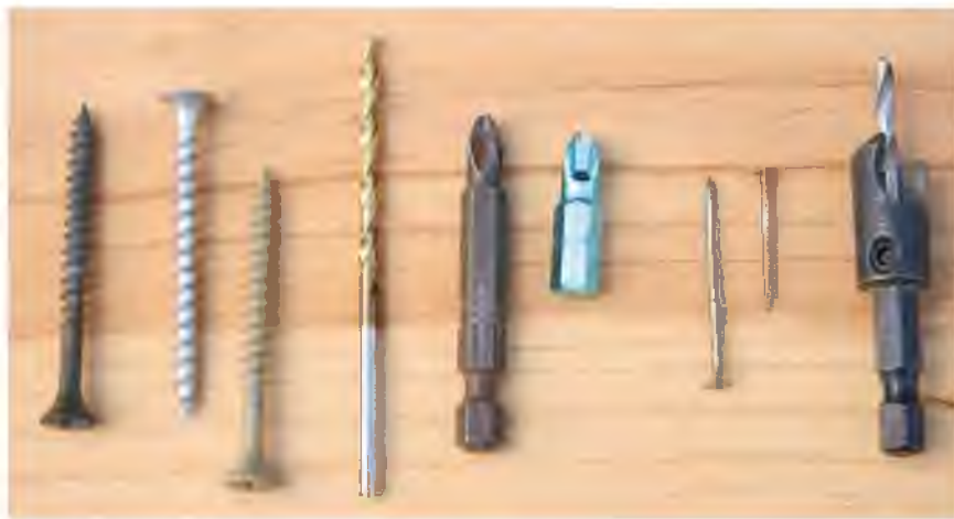
Photo 4 from L to R: Coated deck screws, standard drill bit, long and short screw driver bits, clay coated frame nails and a countersink.
